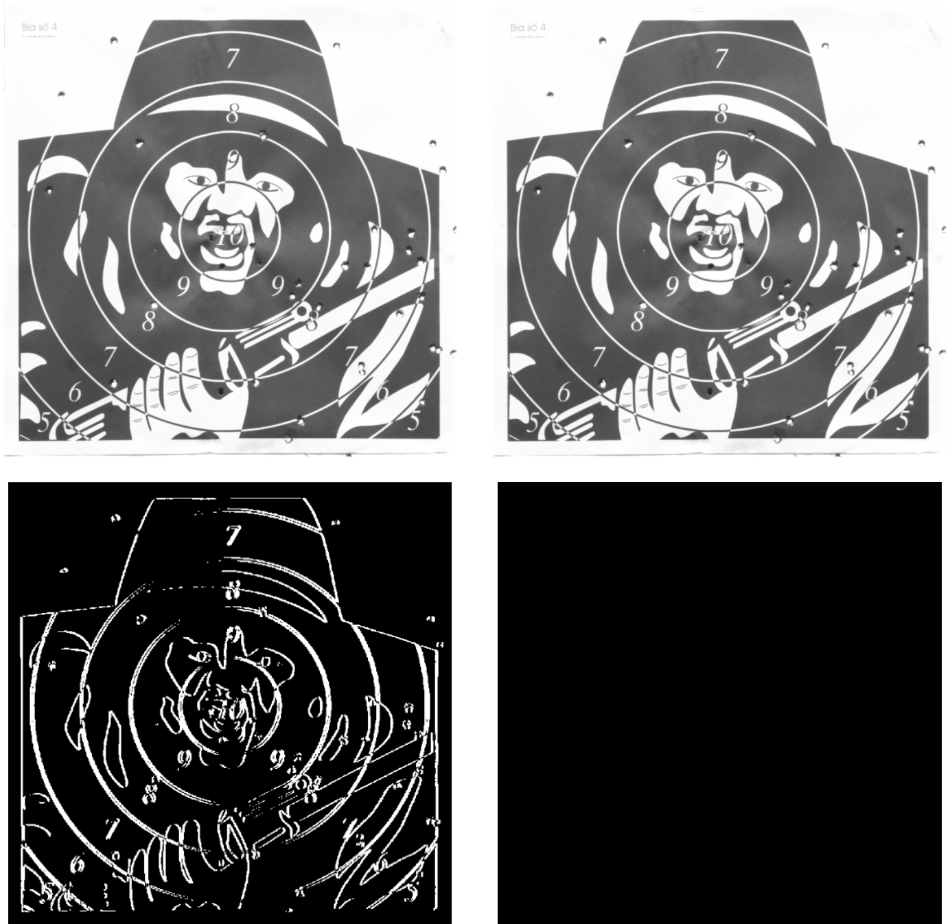
Figure 3. The dense optical flow enabling precise background subtraction even under camera shake. Two consecutive images are on top. With optical flow (bottom right), the current frame is well aligned to the previous frame, preventing differences between two images (bottom left).
