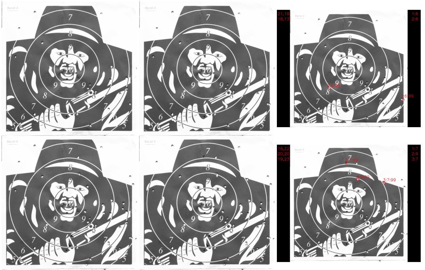
Figure 4. Visualization of complete shooting sessions processed by the proposed system. For each row: (left) first frame of the series (clean target); (middle) final frame after all shots; (right) automatically detected and scored bullet holes overlaid in red on the last image frame
