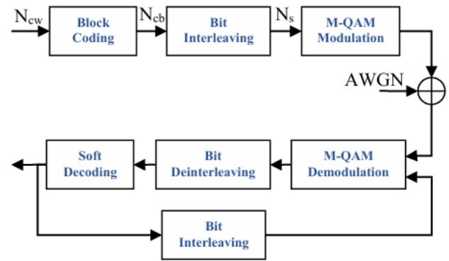
Figure 1. Block-diagram of the BICM-ID system.
