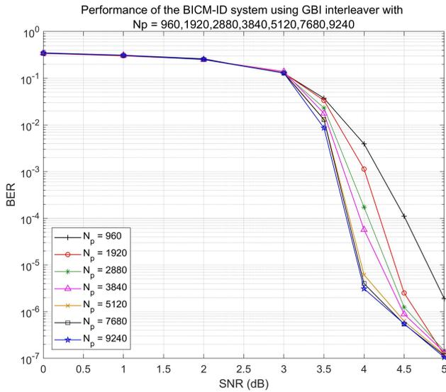
Figure 4. Comparison of the quality of the BICM-ID system using algebraic GBI interleaver with different interleaving lengths  $N_p$ .
