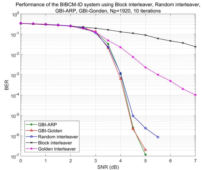
Figure 3. Quality of the BICM-ID system using BI, Rand, and GBI interleaving.
