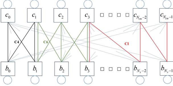
Figure 2. Relations between code and signal nodes of a Bipartite Graph.
